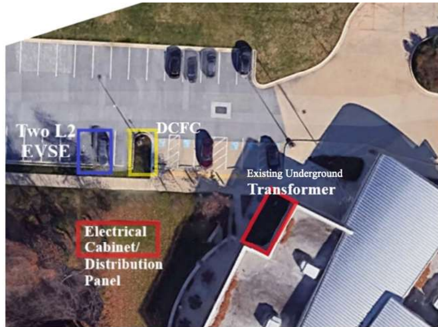
Figure 1. Charging Station Layout.
